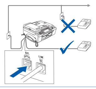
Set the receive mode to 'Manual' if you have an external answering machine. See the section 12 Choosing a Receive Mode on page 14. For more details, see Connecting an external TAD (telephone answering device) in Chapter 7 of the User's Guide.
